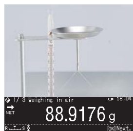
First measure the empty weight.
