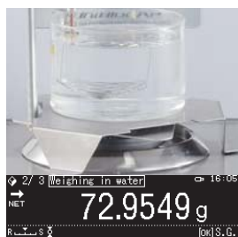
Then place it in the container filled with water, as instructed on the screen.
